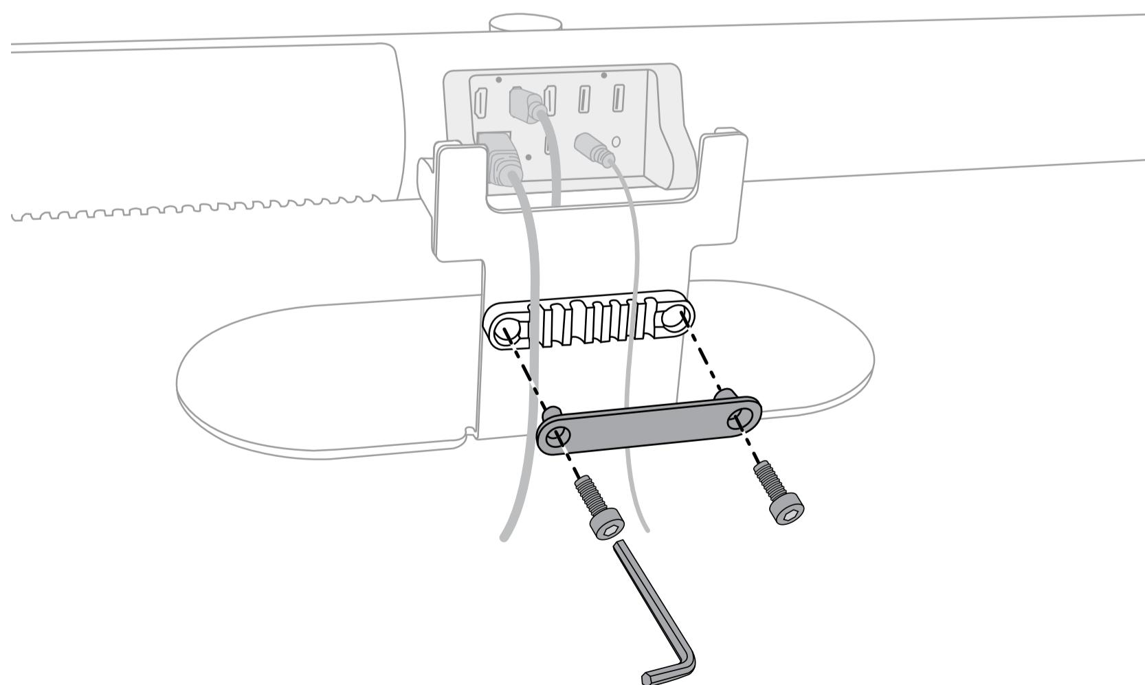
5 Screw the cable cover to the video bar using the supplied screws.
